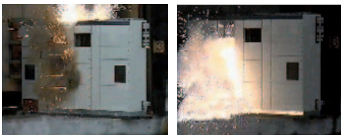
Traditional protection relay systems do not provide fast enough protection in an arc-fault situations.
