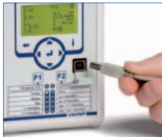
The USB connection is about five times faster than serial communication. Standard USB communication cable is not manufacturer dependent.
